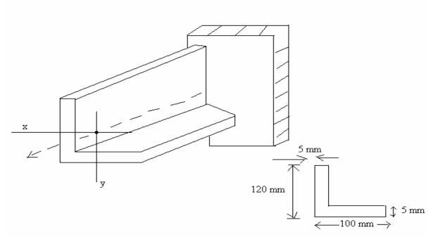
Determine  $I_X$ ,  $I_y$  and  $I_{xy}$  for the unsymmetrical section shown. [16]
